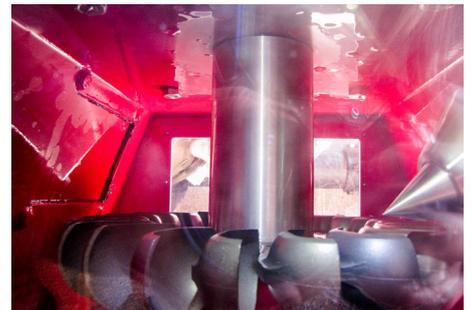
A Turgo turbine and spear valve (to right), built and installed by Hydrolite for TGV Hydro.
